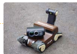
The "moogle" crawling underfloor inspection robot
