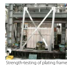
Strength-testing of plating frame
