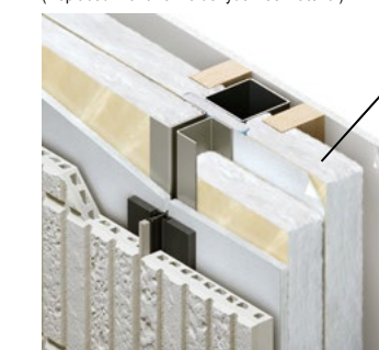
The structure of an external wall of a single-family house
