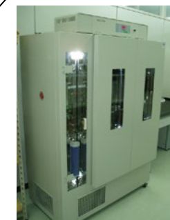
VOC-release measurement using the small chamber method
