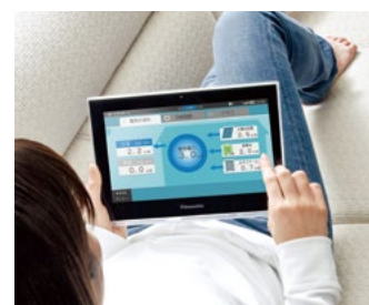
D-HEMS that visualizes energy consumption, etc.
