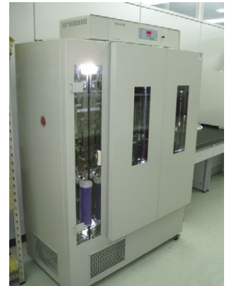
VOC-release measurement using the small chamber method
