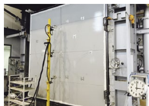
Exterior wall fireproof testing
