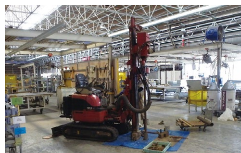
Soil testing (Ryugasaki Plant)
