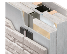
An insulation-backed breathable exterior wall with water and moisture resistance
